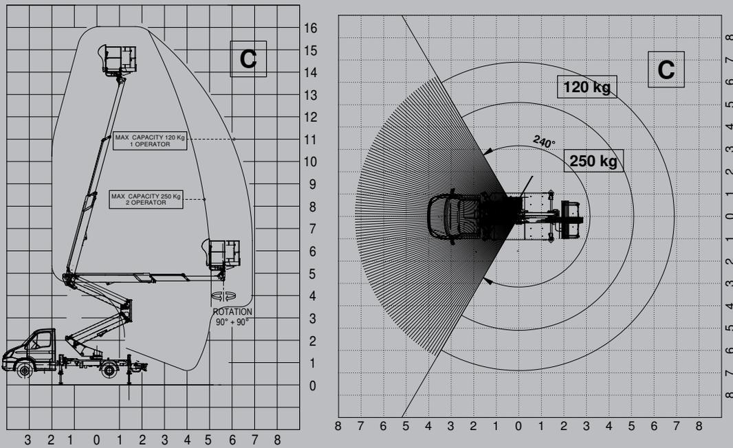
**CROSSBEAMS ONE SIDE FULLY OPENED ONE SIDE CLOSED**
